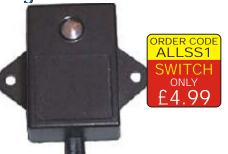
Compact waterproof electronic unit ideal for switching on external lights at dusk (for security) and off again when it gets light (to save electricity). Just install in series with any light bulb rated up to 150W maximum. Not suitable for fluorescent or discharge lights.
