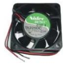
12 VOLT DC Fan Size 60 x 60 x 25mm Type TA225DC. Manufactured in Japan by NIDEC Low Noise Operation. Ball Bearing 12 Volt DC max 90mA polarity protected 300mm Flying Leads 9 cfm Model M33394-16
