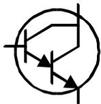
If an NPN Darlington transistor was detected for example, the following message would be displayed:
